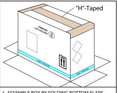
1. ASSEMBLE BOX BY FOLDING BOTTOM FLAPS FIRST, THEN SEALING TWICE WITH 75MM ADHESIVE TAPE IN A 'H'TAPE FASHION.
