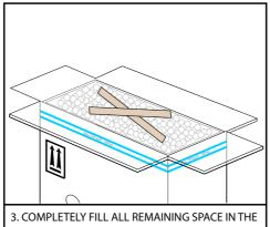
3. COMPLETELY FILL ALL REMAINING SPACE IN THE BAG WITH VERMICULITE, SEALING THE BAG WITH 75MM ADHESIVE TAPE.
