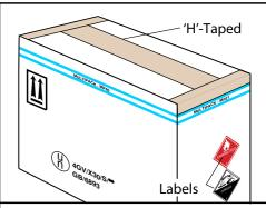
4. CLOSE THE TOP FLAPS OF THE BOX AND SEAL TWICE WITH 75MM ADHESIVE TAPE IN A 'H'TAPE FASHION.
