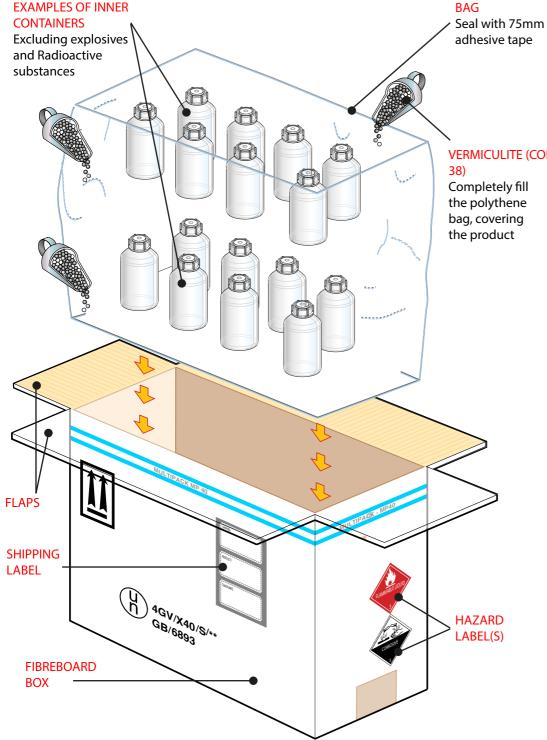
An evenly distributed layer of vermiculite must cover the bottom and top of the packaging spaces.
